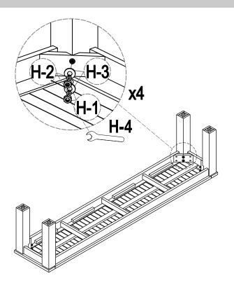
Using a second person to assist you, place Bench Seat Panel (A) upside down on a padded, non-marring surface. Insert bolts on Legs (B) through predrilled holes in corner of apron. Secure bolts with Flat Washers (H-3), Spring Washers (H-2) and Hexagon Nuts (H-1), stacking the hardware in the order as shown. Loosely install hardware on both bolts. Fully tighten using Open Wrench (H-4) after all hardware is installed. Repeat for remaining Legs (B).
